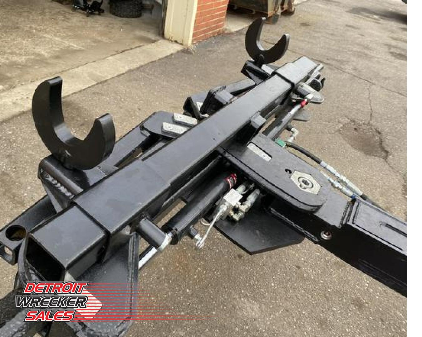
All DWS Crossbars come standard with 2 holes on top of the Crossbars so a client can purchase the Frame Fork Kit later. The holes or provisions for the attachment are there. Giving the operator yet another way to attach the vehicle to the crossbar. Via the Frame, Hitch, Radiator core support or anyway that will allow you to secure your load to the crossbar.
