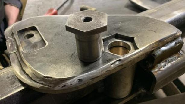
OUR **SUBFRAME ALSO HAS BRONZE OIL-**LITE **BUSHINGS &** OIL SEALS. THE OIL **SEALS KEEP** THE WATER/ **ELEMENTS** OUT & **GREASE IN!**
