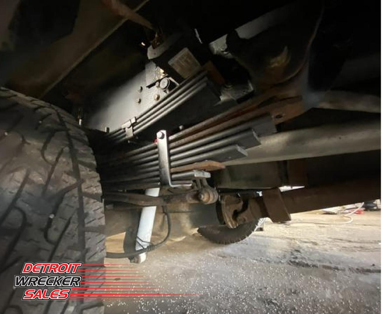
Not all trucks are the same height. Many times the spring shop has put more or less arch in the spring to get us the proper height They also custom make Helper Springs & lower the helper pads. All of these little details add up to a perfect operating procedure.
